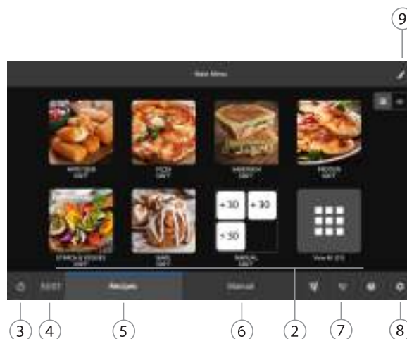
Figure 5: Oven Controls: Group/Temperature Select
