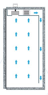
Quadraflow™ Rear Plenum Airflow Design
