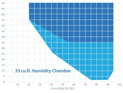
Achievable humidity settings are closely dependent on ambient conditions. Lower humidity may be achieved with accessory compressed air dehumidification system.
