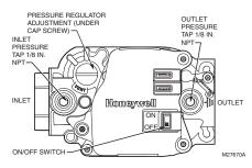
Fig. 4. Top view of gas control.
