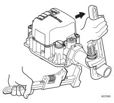
Fig. 3. Proper use of wrench on gas control.
